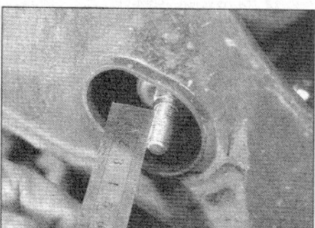
6.9c ... until the length of bolt thread protruding through the drop link nut is as specified
