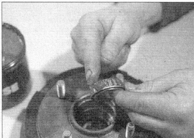
35.5 If the bearings are in good condition, re-pack them with grease of the specified grade
