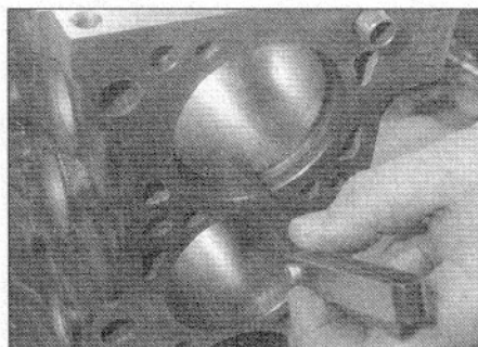
17.4 Checking a piston ring end gap
