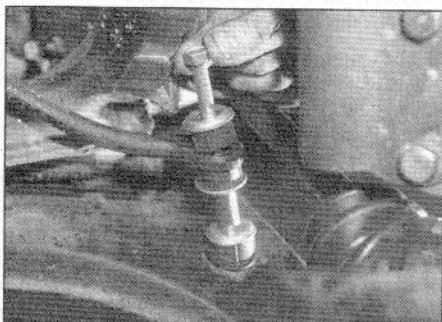
6.8 Refit the drop link components to the end of the anti-roll bar
