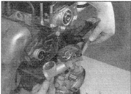
7.14 Fit the coolant pump into position over the gasket, then insert the securing bolts
