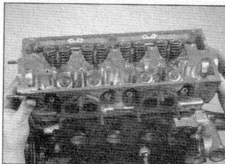
10.19 Lower the cylinder carefully into position ...
