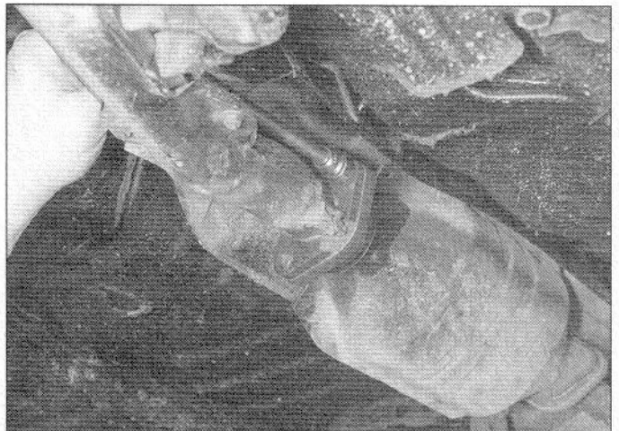
16.7 Removing the front pipe to catalytic converter bolts
