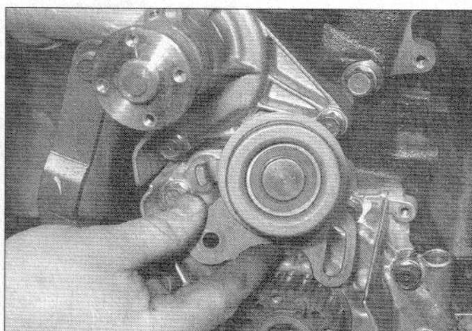
6.10 ... and remove the tensioner pulley
