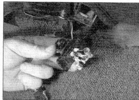
9.33 Remove the screws and withdraw the resistor from the casing
