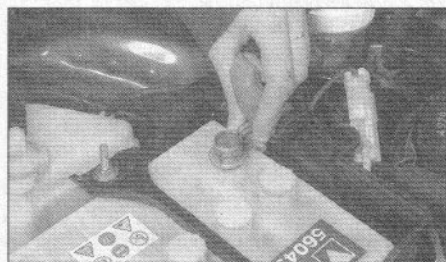
A Check the condition and security of the battery connections
