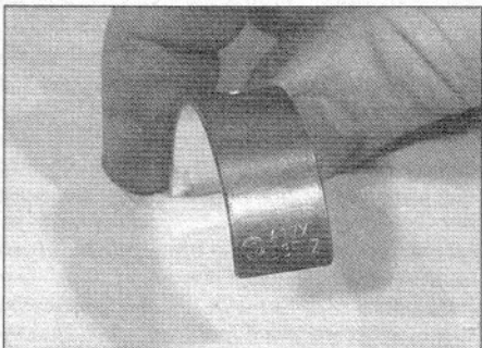
18.2 Typical marking on the back of a bearing shell
