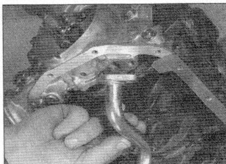
11.6a Refit the pick-up/strainer using a new gasket ...
