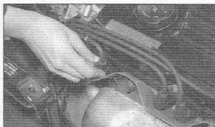
B Check that the spark plug HT leads are securely connected by pushing them onto the plugs
