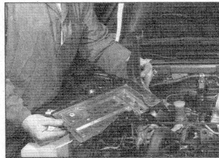
4.5b . . . and, if necessary, unbolt and remove the battery mounting bracket
