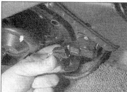
9.32 Unplug the wiring from the resistor at the connector
