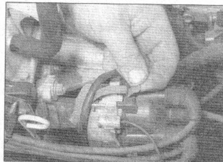
8.3 On 8-valve models release the retaining clips and remove the cap from the distributor
