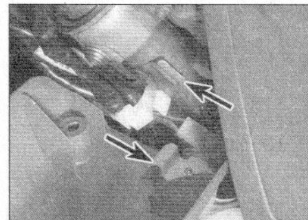
4.8 Engage the metal bracket (arrowed) on the inside of the lower shroud with the mounting bracket on the steering column (arrowed)
