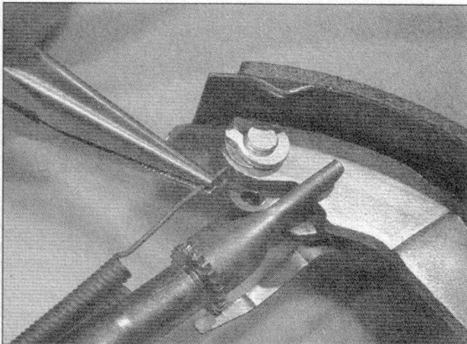
6.53a Hook the upper return spring into the holes at the top of both brake shoes
