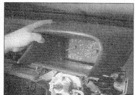
8.4b ... and then disengaging the clips at the upper edge
