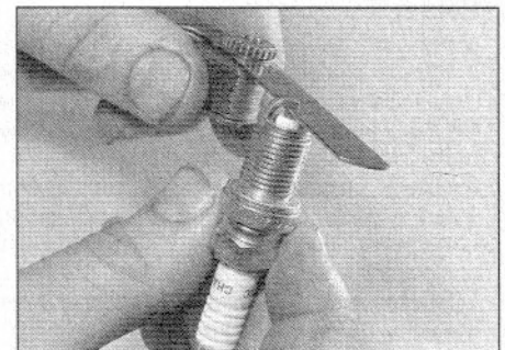
5.9b Measuring the spark plug gap with a feeler blade
