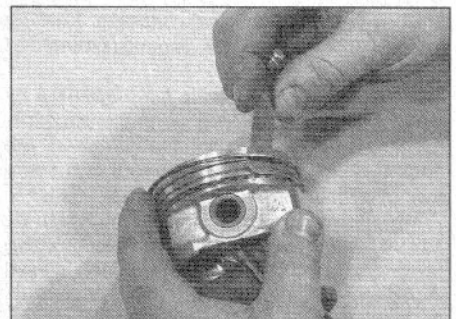
13.2 Using a feeler blade to remove a piston ring
