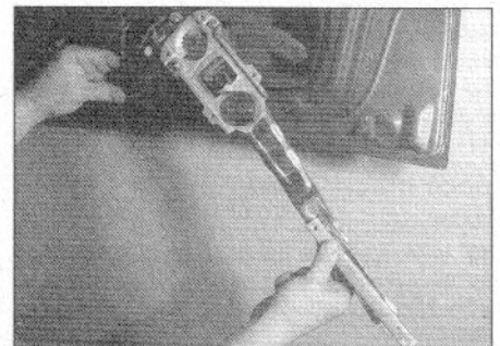
15.10 Manipulate the complete regulator assembly out through aperture in the door (front door with electric windows shown)
