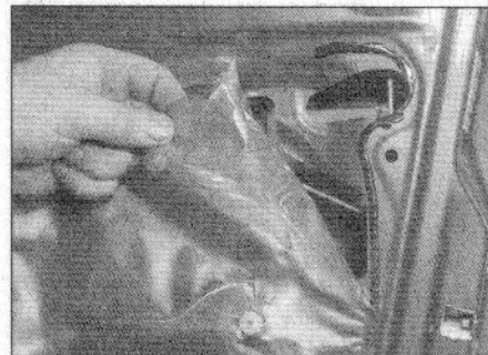
13.8 Peel the plastic sealing sheet away from the door. If necessary, use a sharp blade to split the sealant bead
