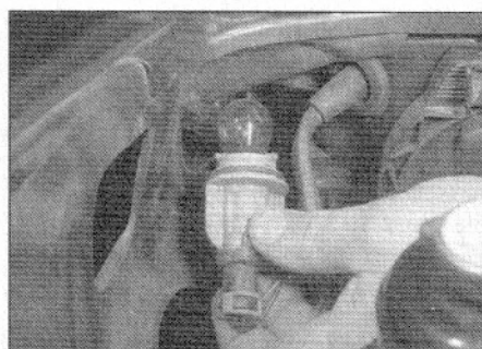
5.18 Twist the bulbholder anti-clockwise and withdraw it from the light unit
