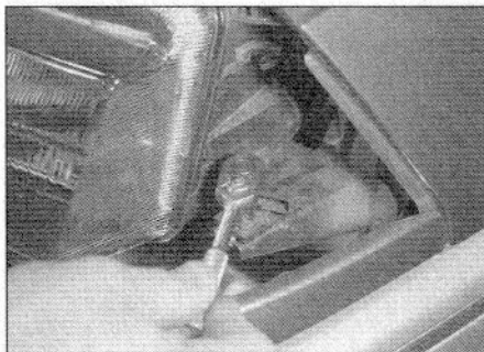
7.4b Remove the headlight unit outer securing screw
