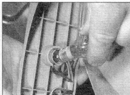
5.34 Release the bulb by twisting it from its bayonet fit holder
