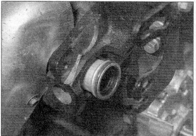
7.13 Fit a new O-ring seal to the end of the water inlet pipe
