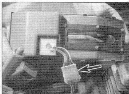
24.2b On models with electric mirrors, unplug the wiring at the connector (arrowed)
