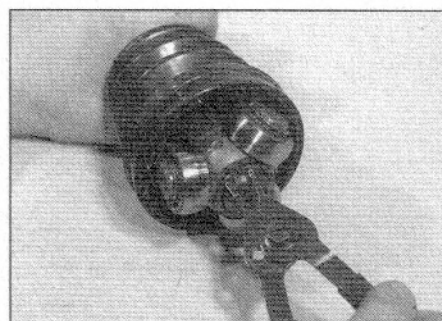
3.6 Remove the circlip from the end of the driveshaft with a pair of circlip pliers
