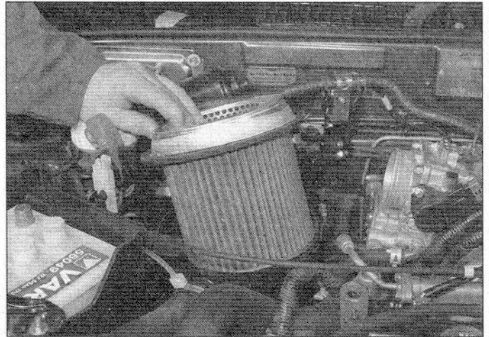
13.15b . . . and lift the off the housing cover and withdraw the filter element
