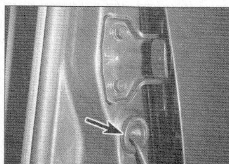
12.4 Prise the wiring harness grommet (arrowed) from the leading edge of the door
