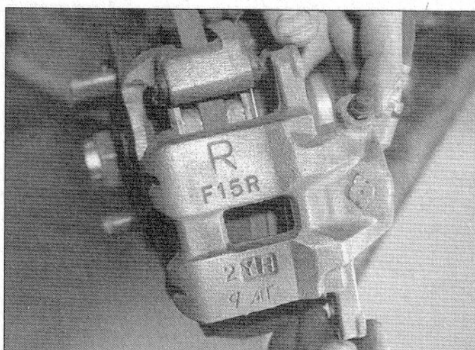
9.7b . . . then remove the caliper from the carrier bracket
