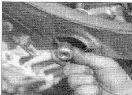
6.9a Pass the drop-link bolt through the suspension lower arm, fit the remaining bushes and washers ...
