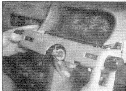
4.13b ... and detach the steering column upper shroud, complete with both switch assemblies
