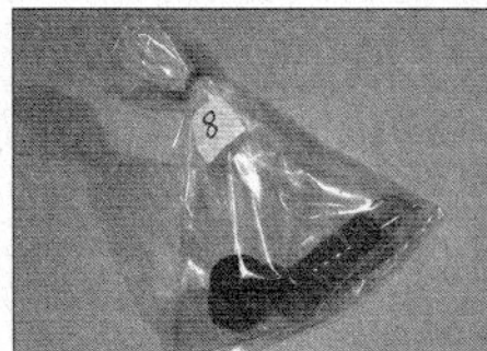
7.6 Place each valve and its associated components in a labelled polythene bag
