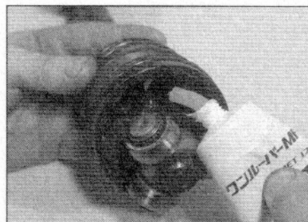
3.23 Slide the gaiter over the tripod joint, then pack the void with grease from the service kit
