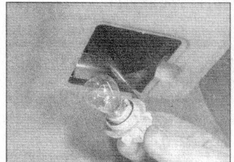
5.31b ... to gain access to the reversing light bulb
